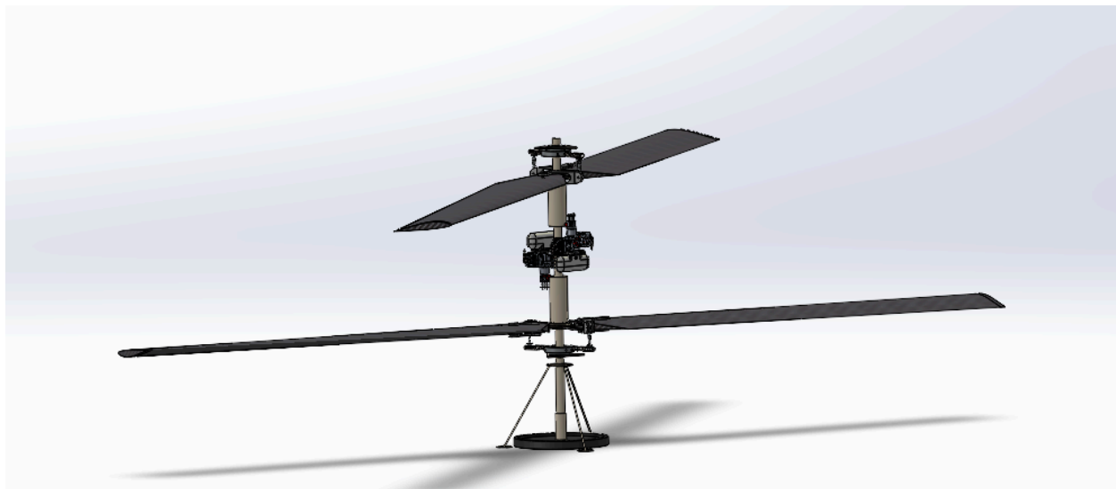
Figure 7: Isometric view of Coaxial blade configuration
