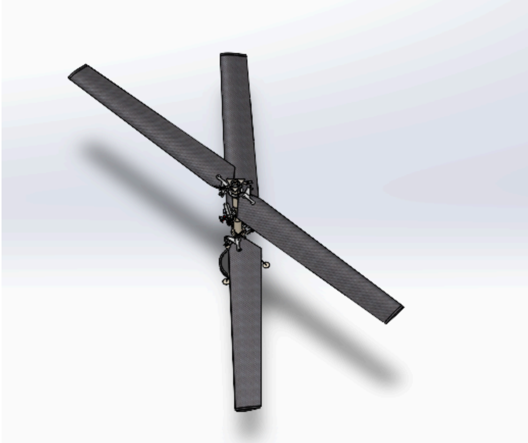
Figure 8: Isometric view of Coaxial blade configuration
